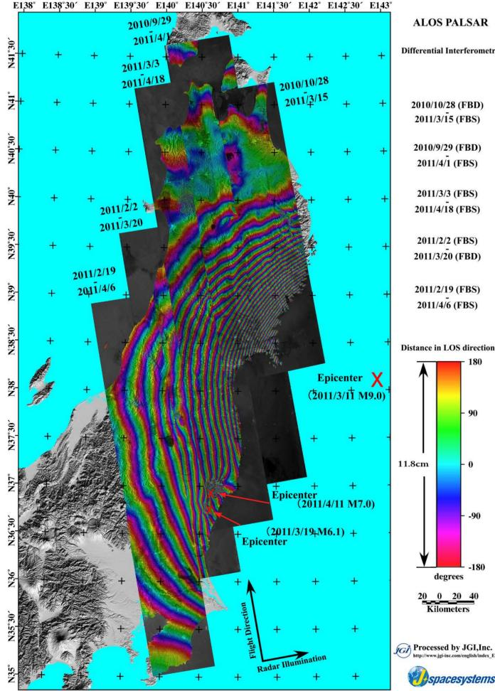
Surface deformation along the direction between the satellite and ground target is shown in color cycle. Northern part (Bluish green $\rightarrow$ Yellow $\rightarrow$ Red $\rightarrow$ Blue, 11.8cm approaching) : Ground uplift Southern part(Blue $\rightarrow$ Red $\rightarrow$ Yellow $\rightarrow$ Bluish green, 11.8cm going away): Ground subside
