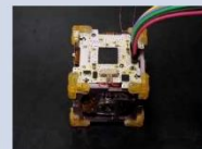
ADCS Module (1 inch cubic 3-Axis RW)
