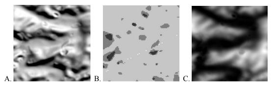
Figure 2. Examples of "pit" artifacts in an ASTER GDEM shaded-relief image (A) that are clearly related to the stack number boundaries (B). Pits typically are less apparent in the normal intensity ASTER GDEM images (C).
