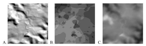
Figure 3. Examples of "mole run" artifacts in an ASTER GDEM shaded-relief image (A) that are clearly related to the stack number boundaries (B). Mole runs, particularly, are less apparent in the normal intensity ASTER GDEM images (C).
